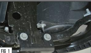
STEP 1 1) From under the rear bumper, take your ZROADZ LED light mount and mock it up into position. This will help you gain familiarity with the mounting orientation. Identify these two bolts that hang the rear bumper on either vehicle corner.
