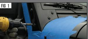
STEP 1 1) Begin by removing the 10 pieces of factory hardware that secure the windshield to the cab of the Jeep.
