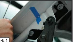
1) Begin by marking the relation between the hinge and hood. Use a piece of tape so you can ensure proper hood alignment when installation is complete.
