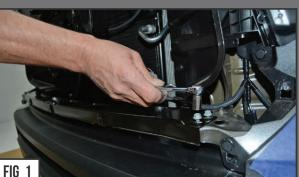
1) With the hood STEP 1 open and grille removed, identify the lower cross member that is secured by (6) bolts, (2) on each side, and (2) in the middle.
