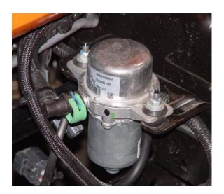
**STEP 1:** Begin by disconnecting the black hose off the front. Disconnect the green hose connecter off of the side along with the black power plug. Unbolt and remove the vacuum canister form the factory mounts.
