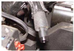
**STEP 3:** Remove the plastic coupling from the large hose coming from the engine and insert the check valve into the end of it.
