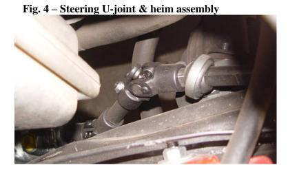
**Step 4:** Reinstall steering components and tighten all necessary setscrews and mounting bolts.
