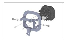
6. Using the included hardware, attach the Type SD bracket to the pod. See the diagram above and make sure the bracket is in the correct orientation. Tighten the bolts down. Do not overtighten or use power tools to torque them down.
