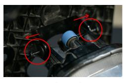
5. Remove the two plastic push rivets shown above that secure the OEM lamp onto the foglight bracket using a trim removal tool (or flat head screw driver).
