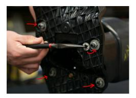
10. Reattach the metal retaining washers.
