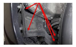
1. Remove the metal brace to gain access to the foglight bracket assembly. Use a 13mm socket and ratchet to remove the four bolts shown above.
