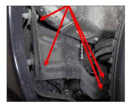
**1.** Remove the metal brace to gain access to the foglight bracket assembly. Use a 13mm socket and ratchet to remove the four bolts shown above.
