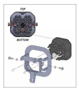
**6.** Using the included hardware, attach the Type SD bracket to the pod. See the diagram above and make sure the bracket is in the correct orientation. Tighten these bolts down all the way.
