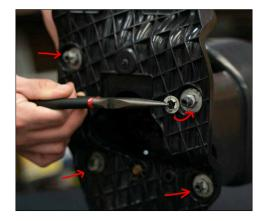
**10.** Reattach the metal retaining washers.
