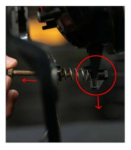
**4.** Remove the adjustment aiming screw using an 8mm socket.
