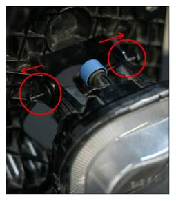
**5.** Remove the two plastic push rivets shown above that secure the OEM lamp onto the foglight bracket using a trim removal tool (or flat head screw driver).
