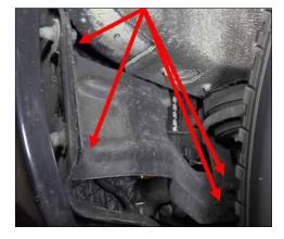
**12.** Finish the installation by reinstalling the metal brace using the four 13mm bolts removed in Step 1.
