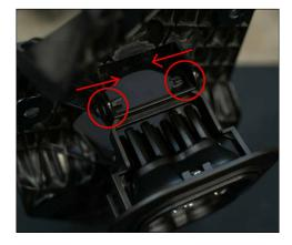
**7.** Install the Type SD bracket onto the factory foglight bracket, by reinstalling the plastic push rivets.
