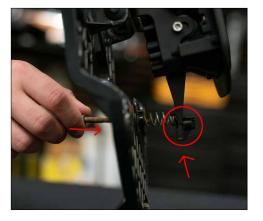
**8.** Reinstall the adjustment screw, spring, and plastic clip to the bottom of the bracket.
