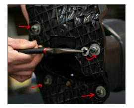
10. Reattach the metal retaining washers.
