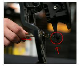
**8.** Reinstall the adjustment screw, spring, and plastic clip to the bottom of the bracket.
