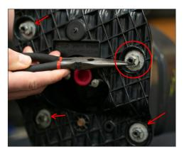
**3.** Set the foglight bracket assembly on a table. Remove the four metal retaining washers using a pick or flathead screw driver. Then remove the four 13mm nuts that secure the front bezel to the foglight bracket.
