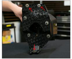
**11.** Reinstall the entire foglight bracket back onto the vehicle using the three 8mm bolts. Use the included wire adapters to connect the pod to the vehicle wiring harness. Test function. If the light does not turn on, try flipping the connector 180°.
