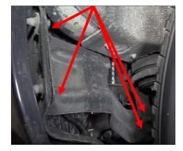
**12.** Finish the installation by reinstalling the metal brace using the four 13mm bolts removed in Step 1.
