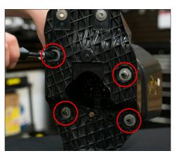
**9.** Reattach the front bezel using the four 13mm nuts. **Do not over tighten.**
