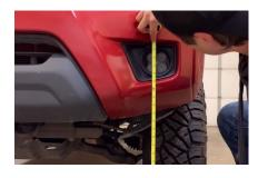
11. On your vehicle, measure the distance between the ground and the center of your SS3 pod. This is your mounting height.
