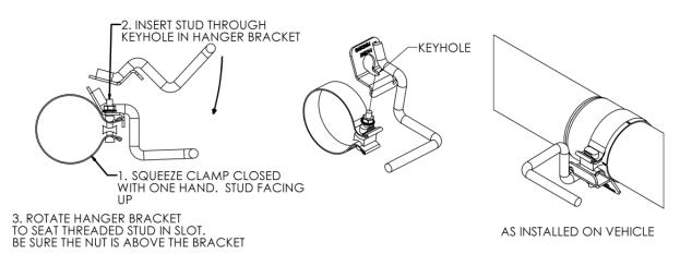
5. Slide the **3**" **Hang Tight<sup>™</sup> Clamp** over the outlet side of the **Muffler**. Position the **Turn Down** and loosely attach it to the **Muffler**. Install the **3**" **Hang Tight<sup>™</sup>** into the existing rubber insulator.
