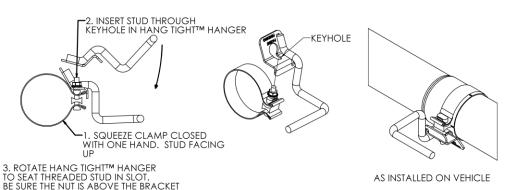
5. Install the hanger assembly from step 4 loosely to the **Extension Pipe** (or **Front Pipe** if the **Extension Pipe** is not required) and place the hanger into the existing rubber insulator. **Refer to Figure 5.**
