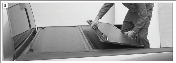
8. Carefully unfold the cover. Position the cover so it is centered side to side and front to back on the truck bed.
