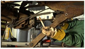
Hold the part up to the frame and take note of its coverage. Mark out a cut line at least 1 inch from the bottom of the frame and trailing arm mount. Ensure that you retain enough material to weld back on to.
