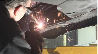
Clean and grind the work area free of rust and debris, revealing bare metal.
