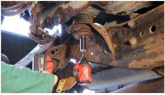
With a jack, lift the body off the frame just enough to remove the bed and cab mount upper bushing.
