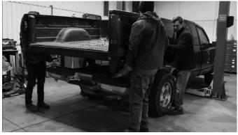
With a 15mm socket, remove the 4 body mount bolts from the body mounts on one side of the vehicle at a time.
