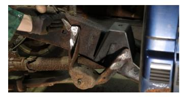
With a 15mm Socket, remove the body and cab mount bolt and bushing.
