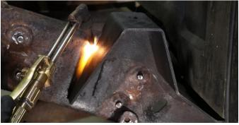
Punch out the spring hanger rivets, and begin cleaning the area free of rust and debris, revealing bare metal.
