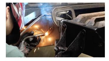
(Re)Install you body mount bolt and bracket. With a jack, raise and lower the body, sliding the bracket to your desired location. Once set, weld it completely to the frame, and remove the jack.
