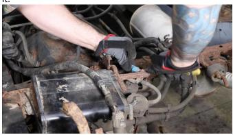
With an exhaust fork, remove the exhaust from the isolators.
