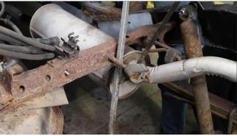
With a 13mm socket, remove the bolt retaining the gas tank strap, and set it aside if not replacing it.
