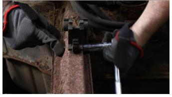
With a 13mm socket and wrench, remove the 4 bolts from each frame rail, freeing the crossmember. Remove the crossmember.
