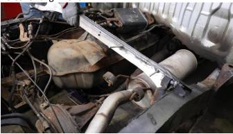
Ensure that the exhaust hangers point to the rear and that the frame holes line up.
