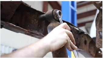
(OPTIONAL): Coat the part with a weld-able primer or other rust inhibitor prior to installation to help prevent or reduce the risk of rust formation.
