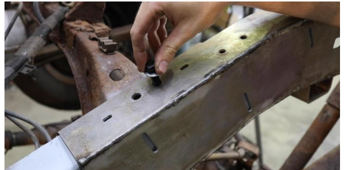
Coat the part and area with a weld-able primer prior
