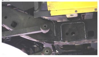
The body mount bracket will need to be removed for this installation. Should you choose to reuse it, be sure to retain as much of the original material as possible.
