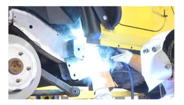
Once secured, use the existing body mount bolt location to help align your old or new body mount bracket to weld it back into place.
