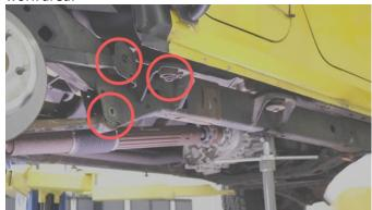
With a 21mm socket, remove the bolts securing both your upper and lower control arms, followed by an 18mm socket to remove the nearby body mount bolt and bushing.
