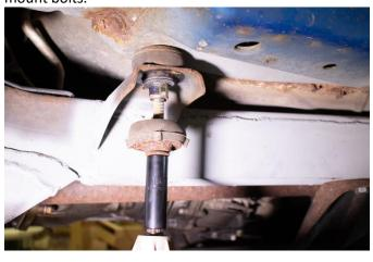
With a hydraulic jack and block or jack stands, push up on the body of the vehicle, near the center, enough so that you can pull the body mount bushing out of its bracket.
