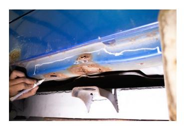
Depending on how you intend to cut, clean the cut zones free of rust and down to bare metal.
