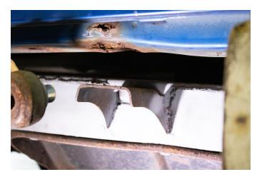
Hold the part up to the body and mark out its installation location, to be cut out later.
