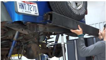
Remove two rear body mount bolts using 16mm.
