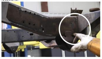
Begin measuring and trimming the stiffener to size.
