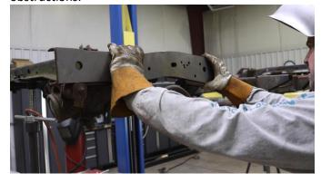
Begin cleaning the frame free of any rust and debris, revealing bare metal.
