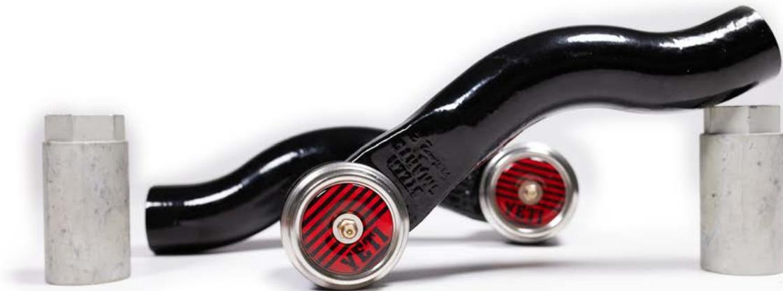
1. Pull boot back and measure current length of outer tie rod from line to center of stud. Note length so you can match the when reinstalling the Yeti XD Outer Tie Rod
