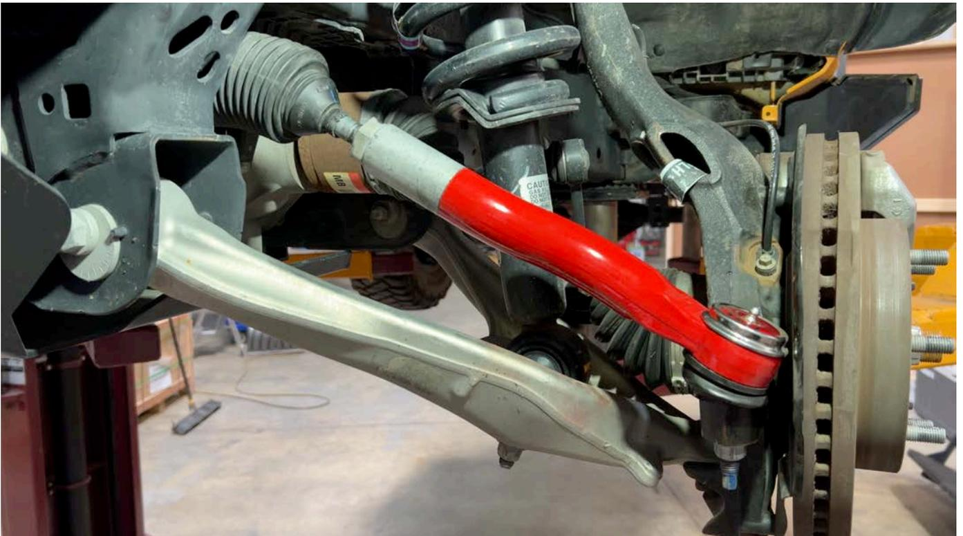
7. Using a 1-1/4 or 32mm crows foot and tighten the inner Jam reinforcement nut to 46 lb ft
