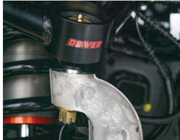
Fig. 18: Reattach UCA to the upright.
