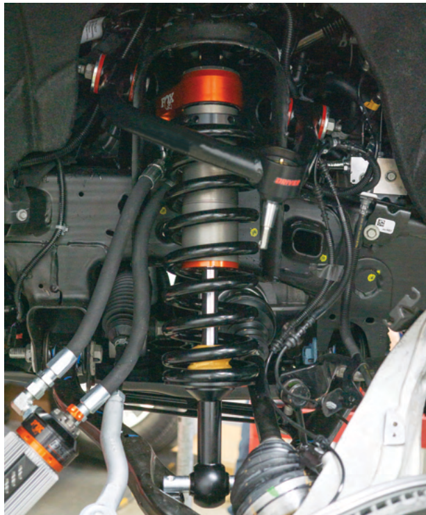
Fig. 13: Driver's side coil-over assembly is featured.
