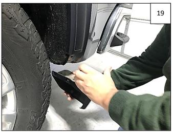
Using a quick jerking motion down and toward you, pry rearward mud guard from vehicle and discard.
