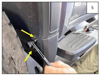
Remove 2 T-15 factory screws from mud guard at inside rear of wheel well. NOTE: It may help to turn the wheel for clearance.
