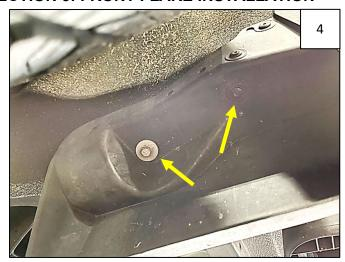
Using a 10mm socket, remove 1 bolt from underside of factory mud guard, at rear of front wheel well. Then use a T-15 Torx bit to remove 1 factory screw. Retain all T-15 Torx screws for later use. Some will be used.
