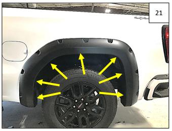
Hold flare firmly on vehicle. Using a grease pencil, mark 7 hole locations through flare onto fender lip.
