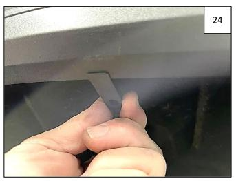
Slide a supplied "U" Clip over plastic lip in 5 locations, centering over marks made in Step 21. Slide a "U" Clip over each Foam Mounting Tab installed in Step 22-23.
