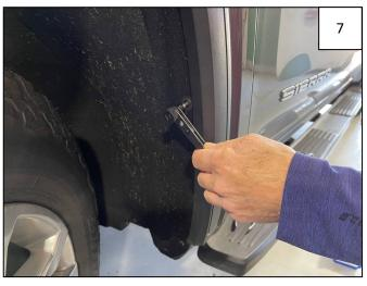
Remove 1 T-15 factory screw from wheel well (above mud guard area).
