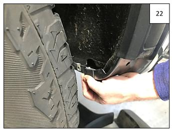
Set flare aside. Peel liner from 2 supplied Foam Mounting Tabs and install over 2 lowermost clip locations marked in Step 21 – on the sheet metal exposed in Step 20.
