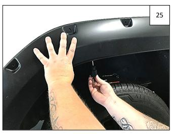
Holding flare firmly on fender, start 7 supplied #10 Truss-Head Screws through holes in flare and into clips installed in Step 24. Ensure flare fit and tighten all screws.
