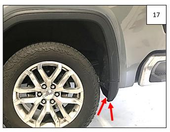
At rear of rear wheel well, remove 2 T-15 bolts from underside of rearward mud guard.
