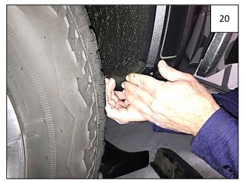
Tuck factory splash shield into fender sheet metal lip at <u>both</u> front and rear of wheel well. The sheet metal lip will need to be accessible for clip installation in Step 24.
