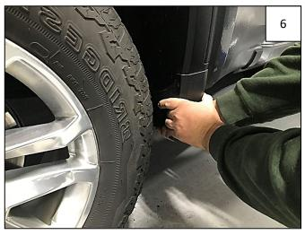
Using a quick jerking motion down and toward you, pry forward mud guard from vehicle and discard.
