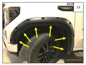
Press flare to fender and tighten all screws.
