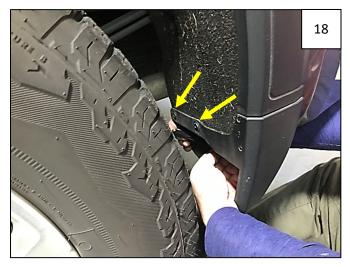
Remove 2 T-15 bolts from mud guard at inside rear of wheel well.
