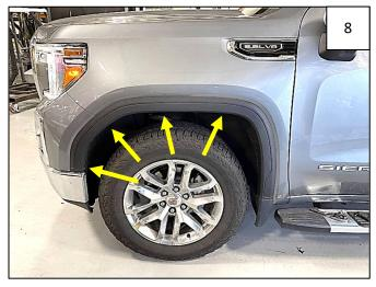
Hold flare firmly on vehicle. Using a grease pencil, mark 4 hole locations through flare onto fender lip.
