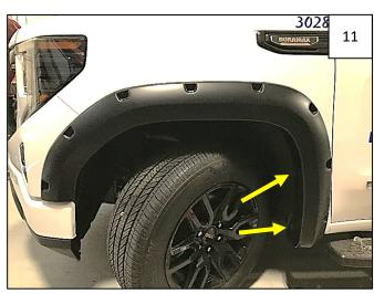
Install 2 factory T-15 Tox screws through rearward holes in flare and into factory holes in fender.
