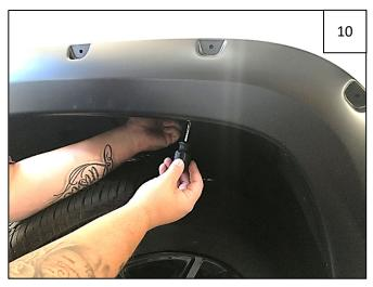
Holding flare firmly on fender, start 4 supplied #10 Truss-Head Screws through holes in flare and into clips installed in Step 9.
