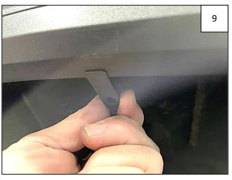
Remove flare from fender and slide a supplied "U" Clip over plastic lip in 4 locations, centering over marks made in Step 8.
