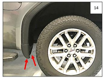
At front of rear wheel well, remove 2 T-15 bolts from underside of forward mud guard.
