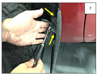
Using a 10mm socket, remove 2 factory fasteners from factory mud flap as shown.
