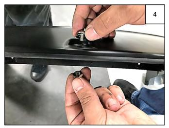
Place a supplied Pocket Nylock Nut over the end of each bolt and tighten using a 1/2" wrench for the Nut and the supplied T-45 Torx Bit for the Bolt. Repeat for all pockets.
