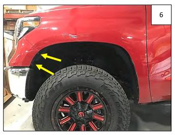
Using a 10mm socket, remove 2 factory fasteners from front of wheel well.
