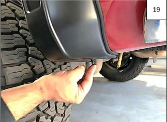
Install supplied 8mm Push-In Retainer through factory hole at rearward underside of flare and into factory hole from which the plastic retainer was removed in Step 15.
