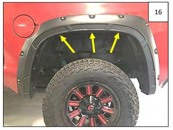
Hold flare on fender, pressing toward vehicle to align holes and start 3 supplied 20mm Hex Screws through the top center holes in flare and into factory holes in fender.
