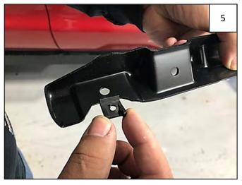
Attach 2 #14 "U" Clips to each Inner Bracket over predrilled holes as shown. **NOTE**: Driver Side Inner Bracket is marked with an "LF" and Passenger Side Inner Bracket is marked with an "RF."
