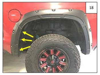
Start 3 supplied 20mm Hex Screws through forwardmost holes in flare and into factory holes in the fender.
