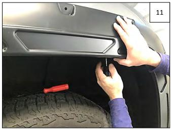
Holding flare firmly on fender, start 4 supplied #10 Truss-Head Screws through holes in flare and into clips installed in Step 10.
