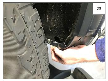
Set flare aside. Peel liner from 2 supplied Foam Mounting Tabs and install over 2 lowermost clip locations marked in Step 22 – on the sheet metal exposed in Step 21.
