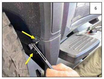
Remove 2 T-15 factory screws from mud guard at inside rear of wheel well. NOTE: It may help to turn the wheel for clearance.
