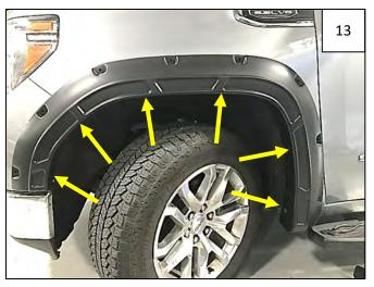
Press flare to fender and tighten all screws.
