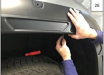
Holding flare firmly on fender, start 7 supplied #10 Truss-Head Screws through holes in flare and into clips installed in Step 25. Ensure flare fit and tighten all screws.
