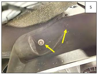
Using a 10mm socket, remove 1 bolt from underside of factory mud guard, at rear of front wheel well. Then use a T-15 Torx bit to remove 1 factory screw. Retain all T-15 Torx screws for later use. Some will be used.
