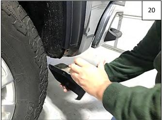
Using a quick jerking motion down and toward you, pry rearward mud guard from vehicle and discard.
