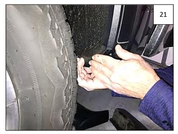
Tuck factory splash shield into fender sheet metal lip at <u>both</u> front and rear of wheel well. The sheet metal lip will need to be accessible for clip installation in Step 26.
