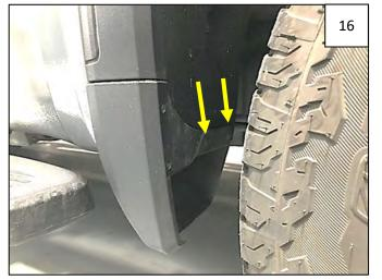
Remove 2 T-15 bolts from mud guard at inside front of wheel well.
