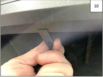
Remove flare from fender and slide a supplied "U" Clip over plastic lip in 4 locations, centering over marks made in Step 9.
