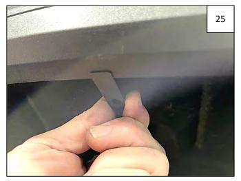
Slide a supplied "U" Clip over plastic lip in 5 locations, centering over marks made in Step 22. Slide a "U" Clip over each Foam Mounting Tab installed in Step 24.
