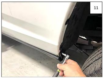
Using an 8mm socket, remove and retain factory screw at front of rear wheel well (this screw holds the underside trim on vehicle at wheel well).
