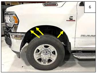
Remove and retain 3 factory screws as shown.
