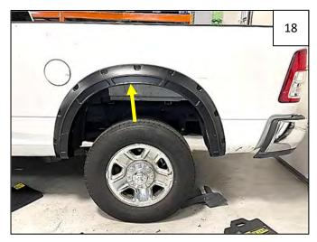
Align flare on fender. Using a Philips screwdriver, start supplied Truss Head Screw through flare and into clip installed in Step 17.
