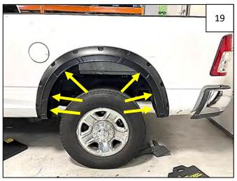
Install 6 retained factory screws through remaining holes in flare and into factory holes in fender.
