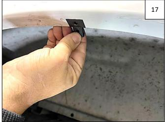
Slide a supplied "U" Clip over the mounting tab centering over the hole made in Step 16.
