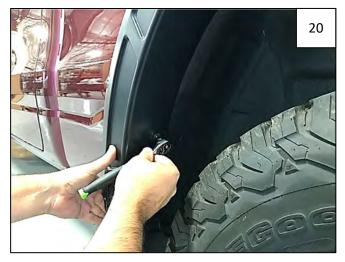
Press inward on flare to apply pressure and tighten all screws.
