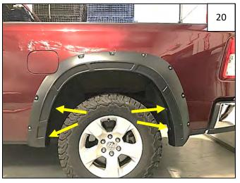
Install 4 retained factory screws through remaining holes in flare and into factory holes in fender.
