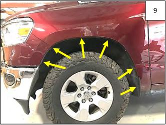
Hold flare to vehicle to note locations of screws to be removed. Remove and retain 6 factory screws from corresponding locations as shown.
