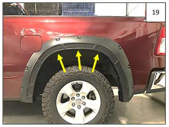
Align flare on fender. Using a Phillips screwdriver, start 3 supplied Truss Head Screws through flare and into clips installed in Step 18.
