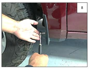
Remove 1 factory screw from center of mud flap. The mudflap will remain on the vehicle – do not remove the other fasteners.
