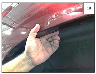
Slide a supplied "U" Clip over each Mounting tab, centering over holes made in Step 17 (3 places).
