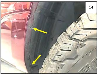
Using an 8mm socket, remove and retain 2 factory screws at front of rear wheel well.
