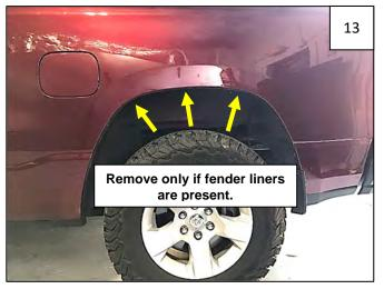
*If vehicle is equipped with fender liners*, remove 3 factory screws at top of fender. If vehicle is not equipped with fender liners, proceed to Step 14.
