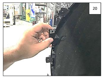
Align slotted hole in bracket with hole in inner fender liner (screw removed in Step 18). Bracket should be at a right angle pointing up with "U" Clip installed in Step 19 at the top.
