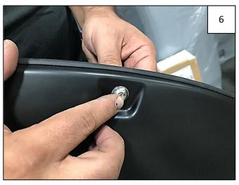
Insert each Bolt/Washer combination through pocket holes in flare, Bolt head and Washer on the outside.
