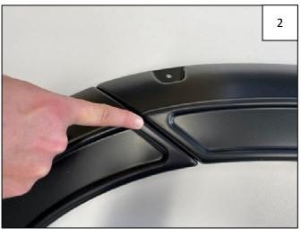
Before tightening, make sure that molded flare features are aligned. Tighten screws using #2 Phillips driver.
