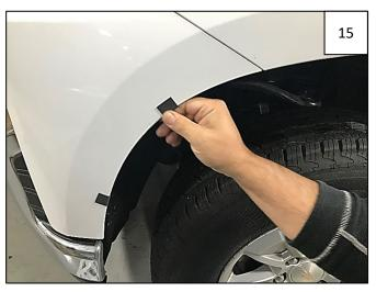
Peel liner from a supplied Foam Tab and center tab over each mark made in Step 14, folding over wheel well lip.
