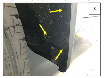
Using a T15 Torx bit, remove 3 factory fasteners indicated by arrows holding the factory mud flap on. Retain all screws.
