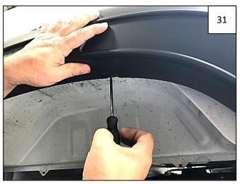
Start 3 supplied Truss-Head Screws through upper holes in flare and into clips installed in Step 29. Apply pressure to flare towards vehicle body at each fastening point and tighten all fasteners.
