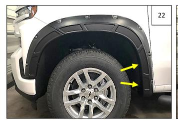
Align flare on vehicle and start 2 factory T15 Torx screws at bottom rear of wheel well as shown.
