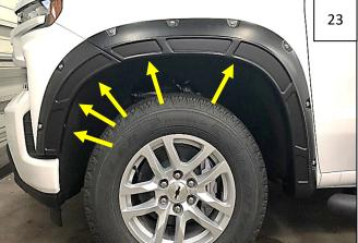
Start 5 supplied Truss-Head Screws through holes in flare and into fender as shown. Apply pressure to flare towards vehicle body at each fastening point and tighten all fasteners.
