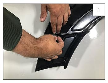
Install extension pieces to main front flares using 2 supplied #8 Speed Clips and #8 Truss Head Screws per side.
