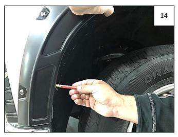
Align flare on vehicle and mark 2 forward hole locations with a grease pencil (upper and lower holes).
