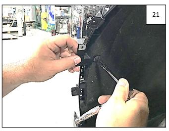
Reinstall screw removed in Step 18 through slotted hole in bracket and into hole in fender liner. Tighten this screw.
