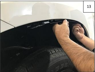
Install Inner Bracket using 2 T15 Torx screws retained in Step 12. Tighten both fasteners. **NOTE:** Driver Side bracket is marked with LH, Passenger Side is RH.
