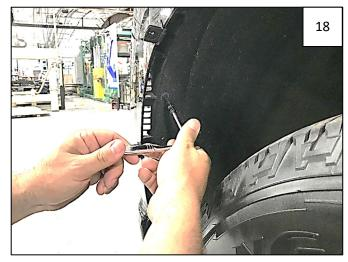
Remove T15 Torx screw from inner liner fender (located between the 2 clips installed in Step 17) as shown.
