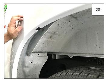
Peel liner from a supplied Foam Tab and center tab over each mark made in Step 26; fold each tab over lip of wheel well.
