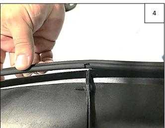
When you come to the jointure of the flare and extension piece, cut a notch in the back of the edge trim.
