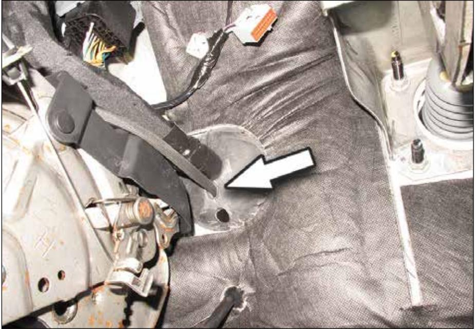
**8.** Plug the OBDII cable into the OBDII port under the dash (**Figure 10**).
