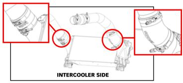
**12.** Once your new boost tubes are pre assembled, they can be loosely installed in the truck. Figure 12
