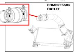
**Figure 11c** Clamp Assembly Positions Roth Sides Lower
