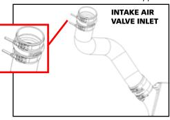
**Figure 11b** Clamp Assembly Positions Passenger Side Upper
