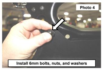
4. Install the remainder of the supplied bolts, nuts and washers across the lower door, and reinstall stock hardware with the door cover. **See Photo 6**.
