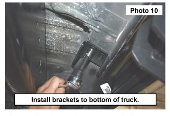
13. When steps and rail are in the desired location, go back and tighten all hardware using a 13mm socket/wrench.
