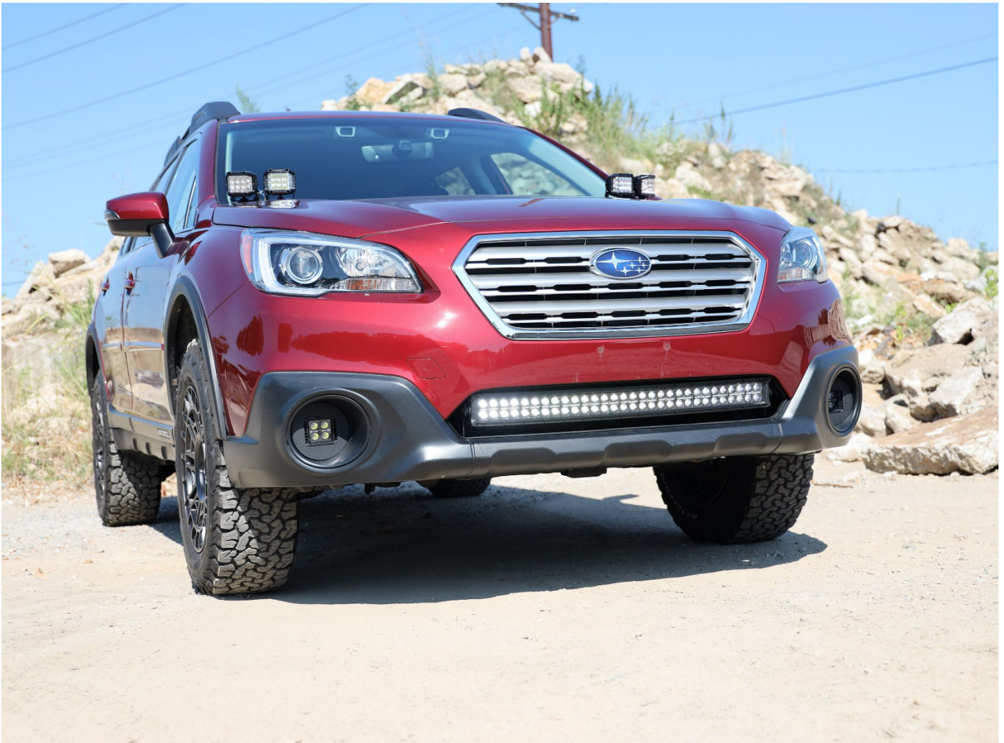
Shown with 30" bumper light, cube fog light replacement, and dual ditch light mounts.
