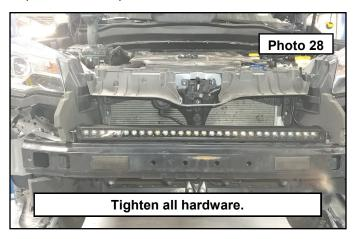
7. Wire the lights accordingly using the provided harness. Reinstall the bumper cover in the reverse order of the disassembly steps.
