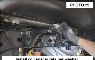
Install coil spacer retainer washer.
