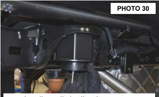
Install supplied coil spring spacers.
