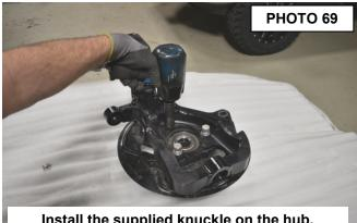
Install the supplied knuckle on the hub.
