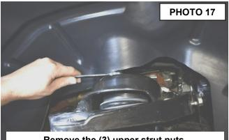
Remove the (3) upper strut nuts.
