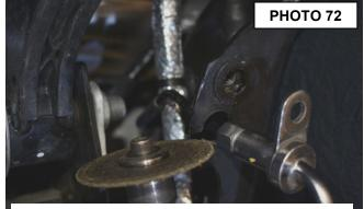
Cut opening in brake line mounting hole.
