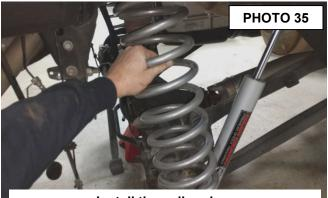
Install the coil spring.
