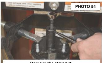
Remove the strut nut.
