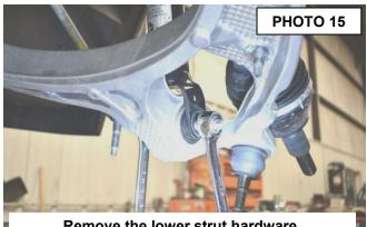
Remove the lower strut hardware.
