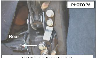
Install brake line in bracket.
