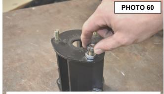
Install the studs in the strut spacer.
