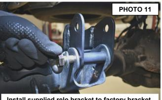
Install supplied relo bracket to factory bracket.
