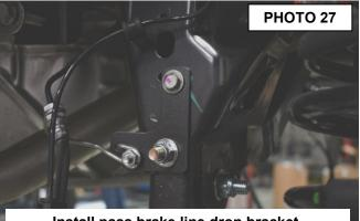
Install pass brake line drop bracket.
