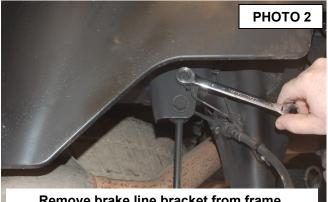
Remove brake line bracket from frame.
