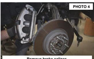
Remove brake caliper bolts.
