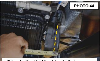
Trim plastic shield for driveshaft clearance.
