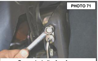
Remove brake line from frame.
