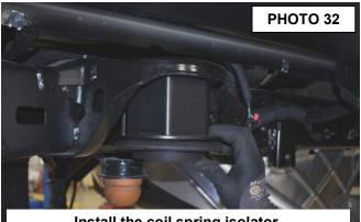
Install the coil spring isolator.
