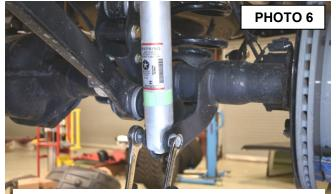
Remove lower shock hardware and shock.
