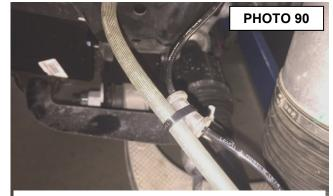
Secure the ABS wire to the brake line.
