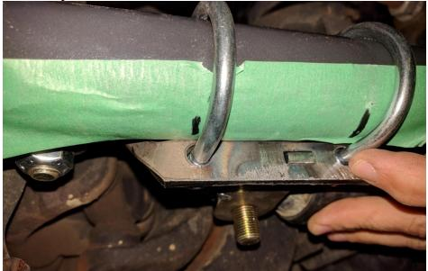
Figure 4. Clamp Centered on Tie Rod
