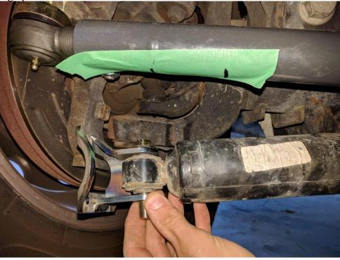
Figure 3. Correct Orientation of Steering Stabilizer Clamp
