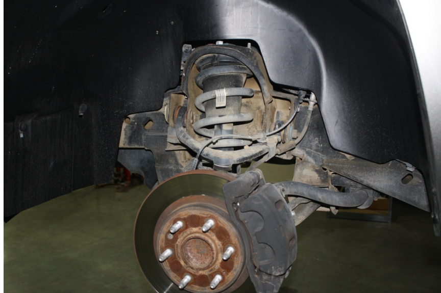
Figure 1: ready to unbolt the strut
