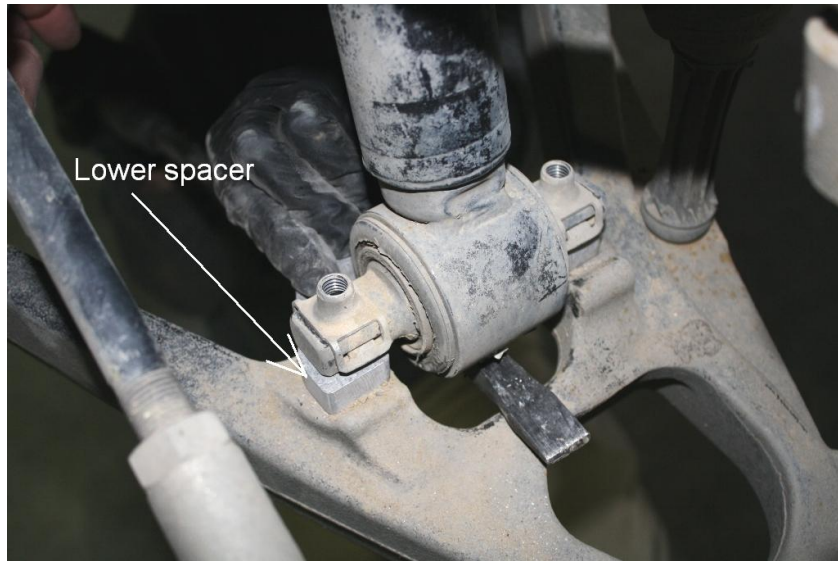
Figure 6: Re-installing lower end of strut with spacer.
