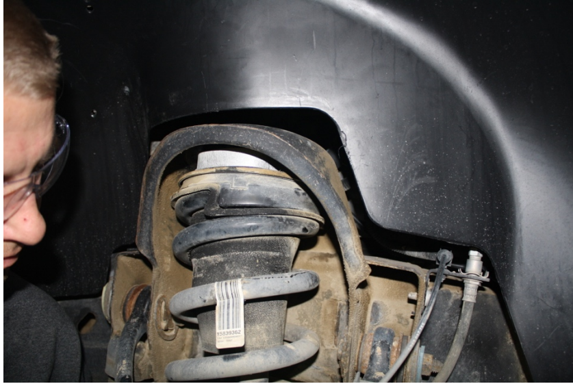
Figure 5: bolting upper end of strut back into the frame
