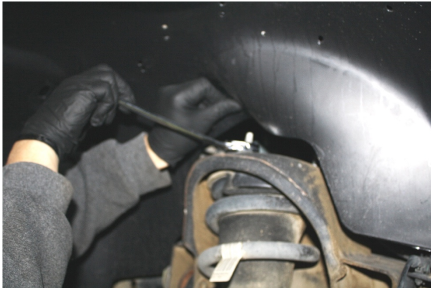
Figure 2: removing upper strut fasteners
