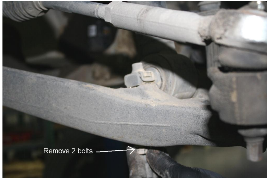
Figure 3: Remove 2 bolts on bottom of lower arm
