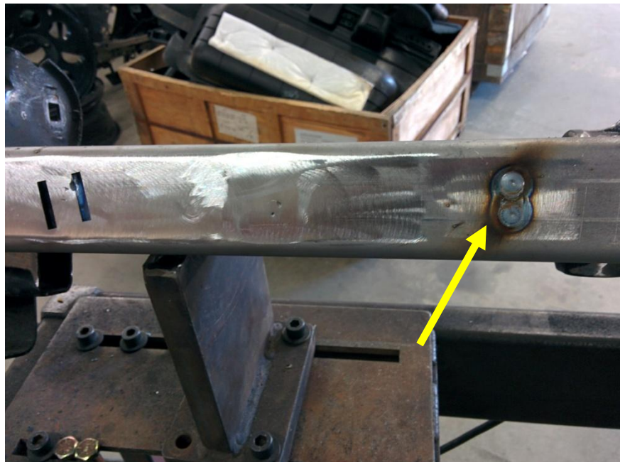
Figure 15. Center Plate Tops Welded to Truss
