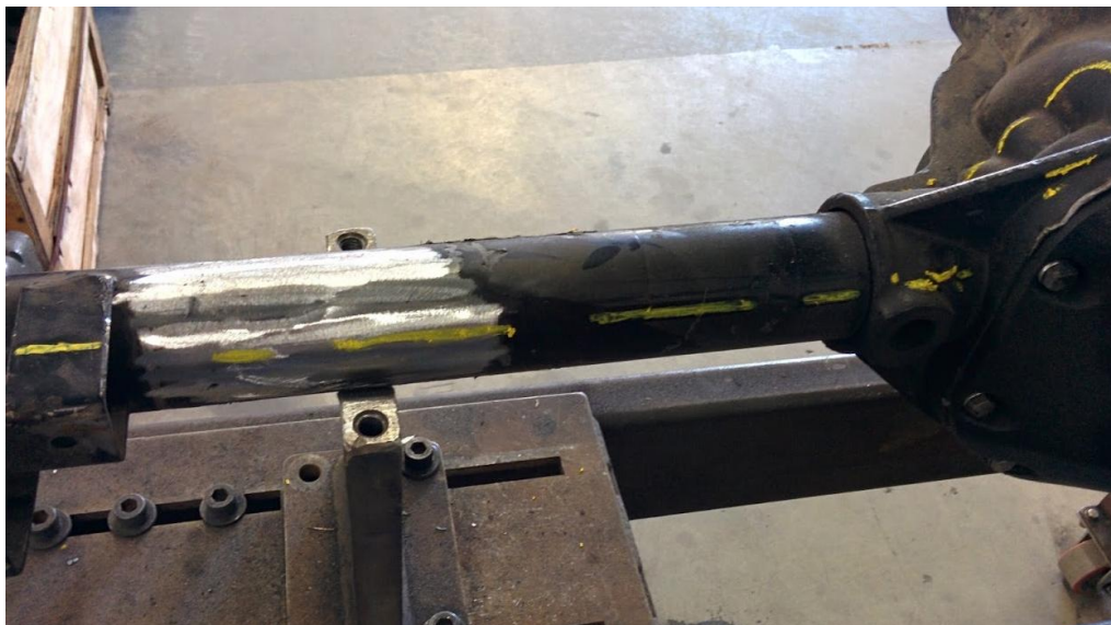
Figure 5. Truss Removed, Showing Areas to Clean
