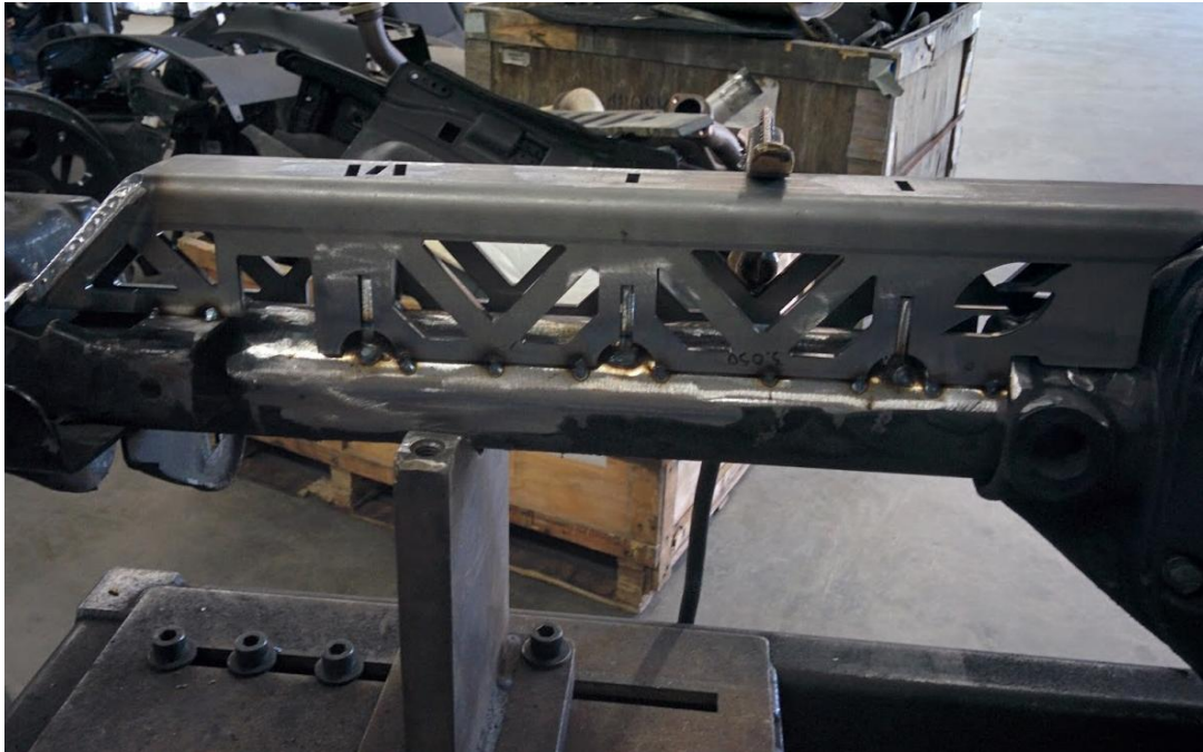
Figure 12. Front Side of Axle Truss Tacked
