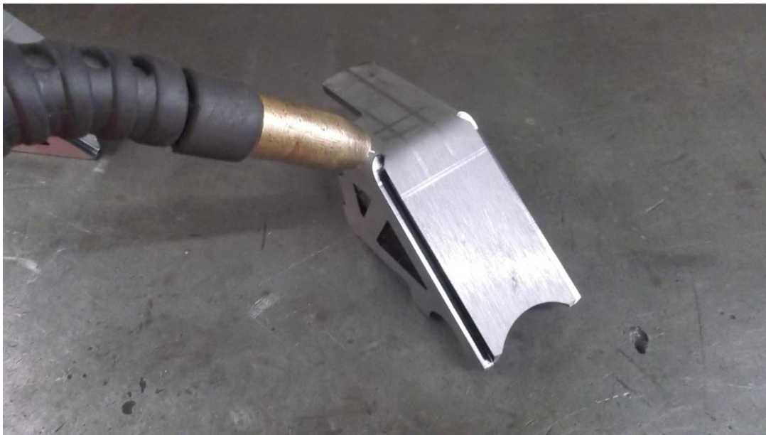
Figure 7. Welding Truss Bend Seams
