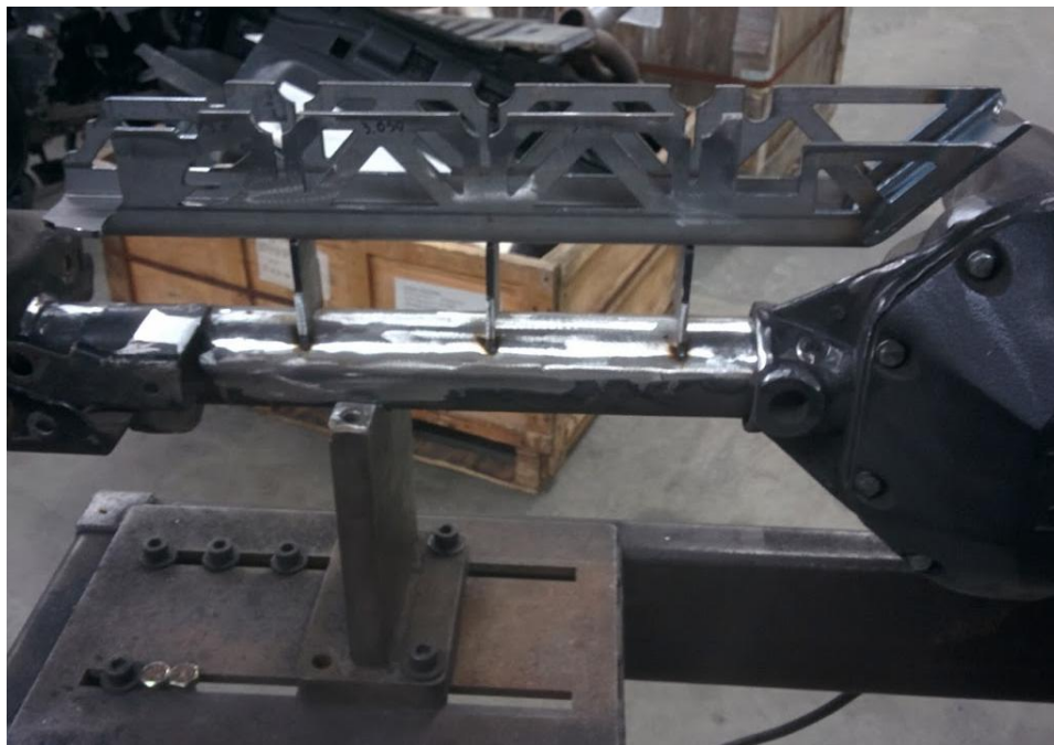
Figure 11. Truss Used as a Fixture
