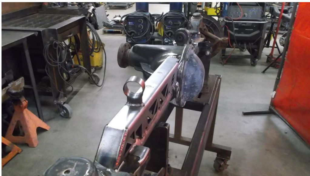
Figure 19. Bushing Mount Welded to Truss
