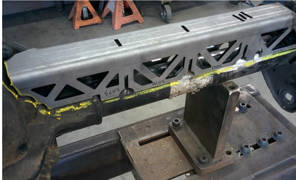
Figure 4. Passenger Side Truss Test Fit and Marked
