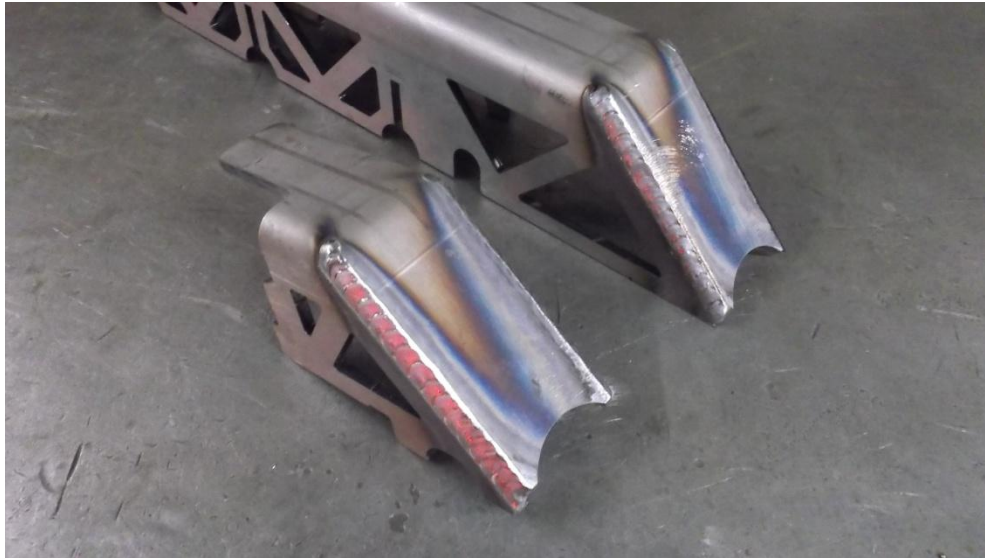
Figure 8. Welded Truss Bend Seams
