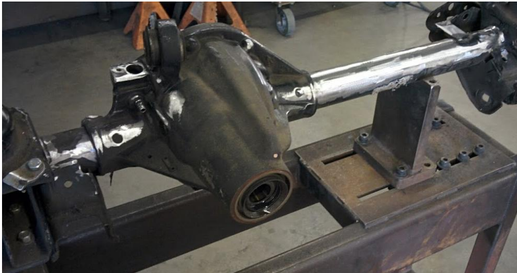
Figure 6. Axle Cleaned to Bare Metal
