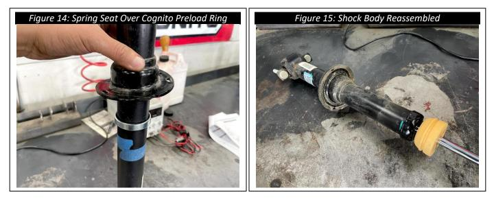
**16.** Reassemble the shock body and the strut assembly. Make sure to align the markings created in the prior step before tightening the center nut on the top of the strut assembly. Torque to **33 ft-lbs**.
