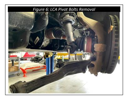
8. Remove the strut from the vehicle. Remove the 3x nuts on top of the strut to free the strut from the frame.
