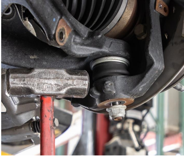
Figure 10: Loosen Lower Ball Joint
