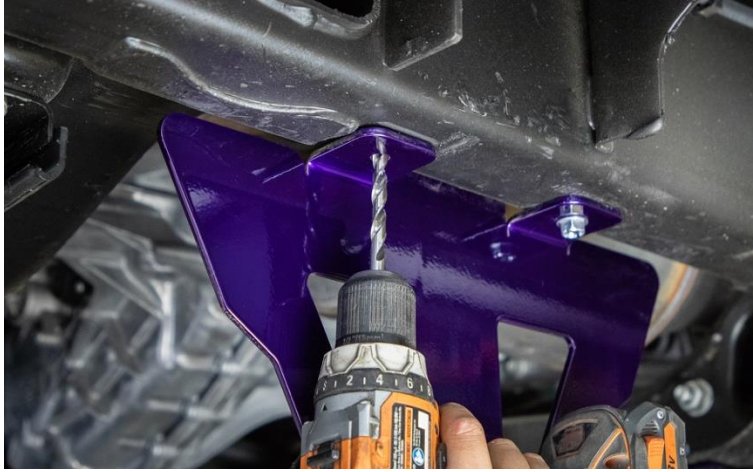
Figure 68: Torsion Bar Drop Bracket Drilling
