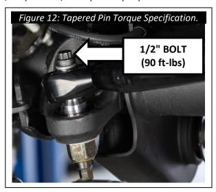
**10.** The following instructions are to adjust the steering wheel back on center. Make sure the vehicle is in park with the emergency brake activated, then start the engine. Loosen drag link adjuster sleeve and adjuster lock, slide the lock out of the way. Rotate the drag link adjuster in the appropriate direction to center the steering wheel.
