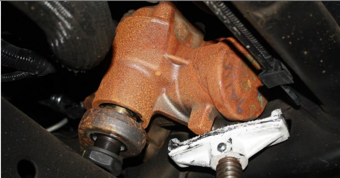
Figure 4: Support the Steering Box with a Jack
