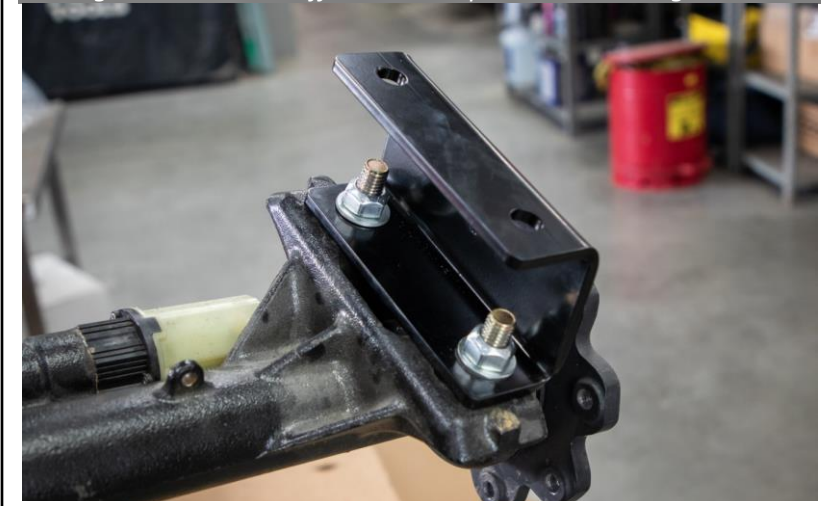
Figure 29: Mount Differential Drop Bracket Passenger Side
