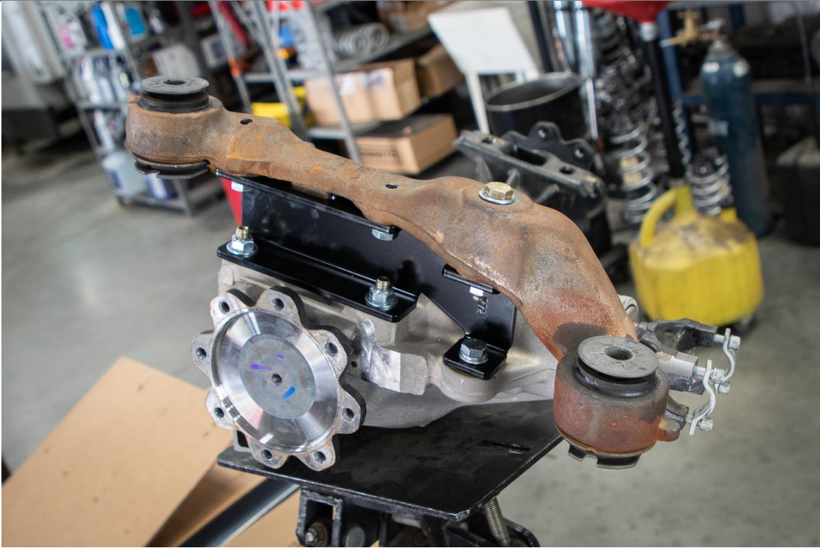
Figure 28: Mount Differential Drop Bracket Driver Side
