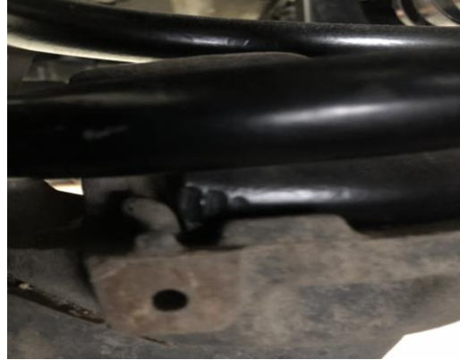
Figure 14B: Bottom Spring Pig-tail Orientation
