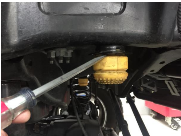
Figure 10A: OE Bump Stop Spacer
