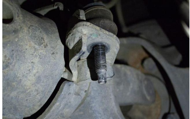
Figure 7B: OE Sway-Bar End Link, Nut Removed
