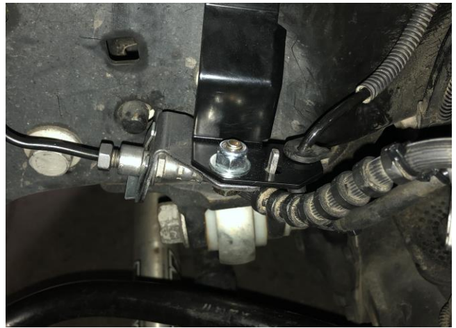
Figure 6: Passenger Side ABS Line Routing
