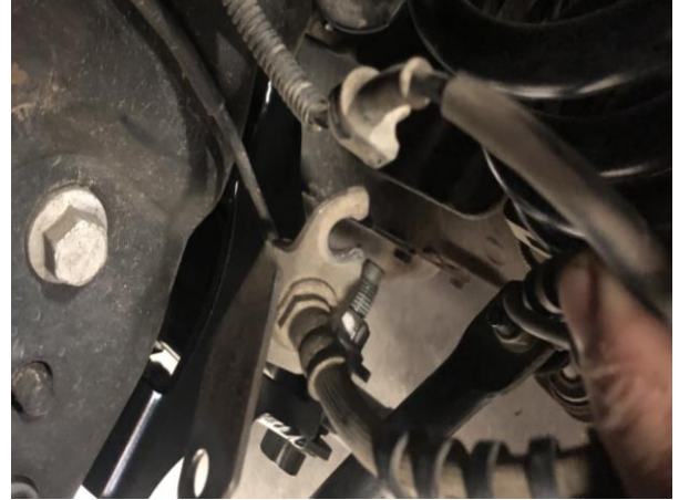
Figure 2B: Driver ABS Line Removal
