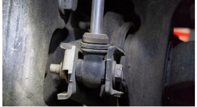
Figure 16B: Front Lower Shock Mount Installed
