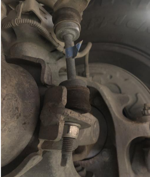
Figure 7A: OE Sway-Bar End Link
