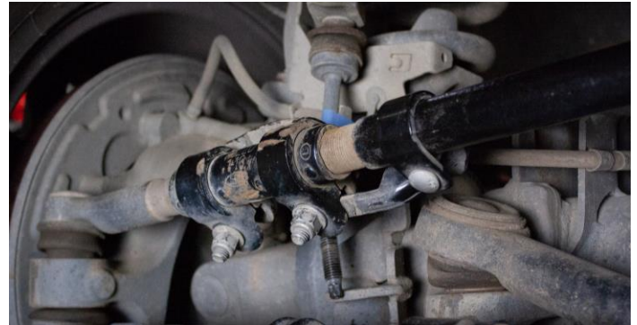
Figure 17B: Steering Link Adjuster Secure
