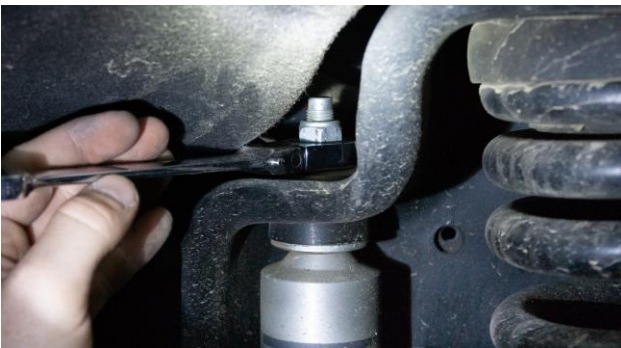
Figure 8A: Front Shock, Top Mount
