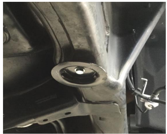
Figure 10B: FSD Bump Stop Spacer Hardware
