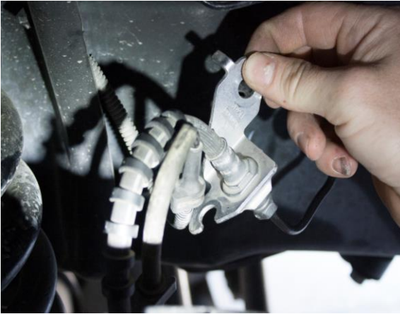
Figure 2A: Passenger ABS Line Removal
