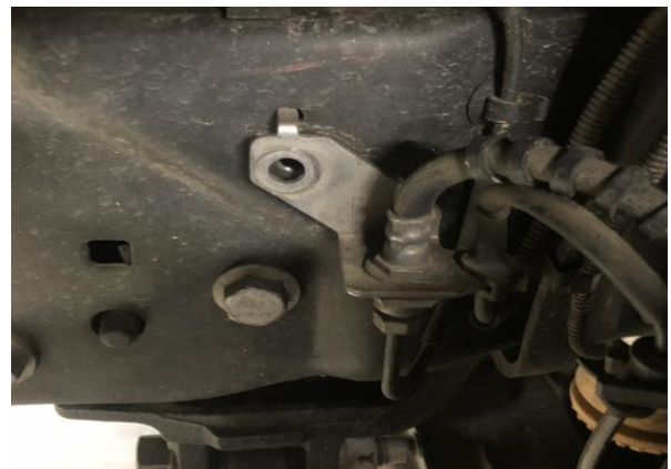
Figure 1B: OE Brake Line Bracket, Bolt Removed
