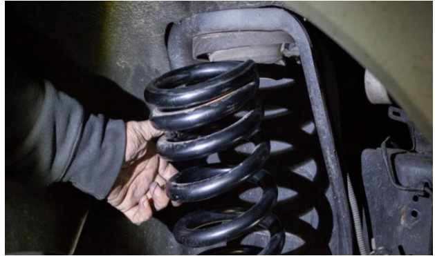
Figure 9B: Spring Removal
