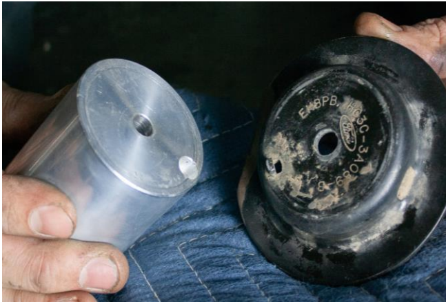
Figure 12: Bump Stop Spacer Alignment
