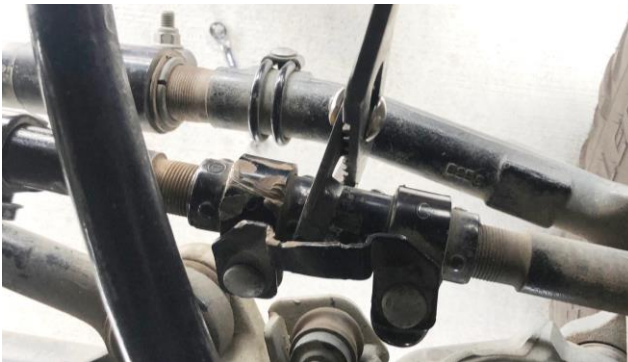
Figure 17A: Steering Link Adjustment
