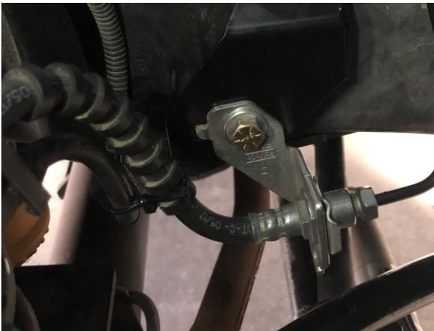
Figure 5: Diver Side ABS Line Installed
