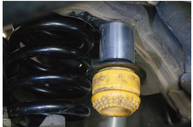
Figure 13: Bump Stop Spacer Orientation
