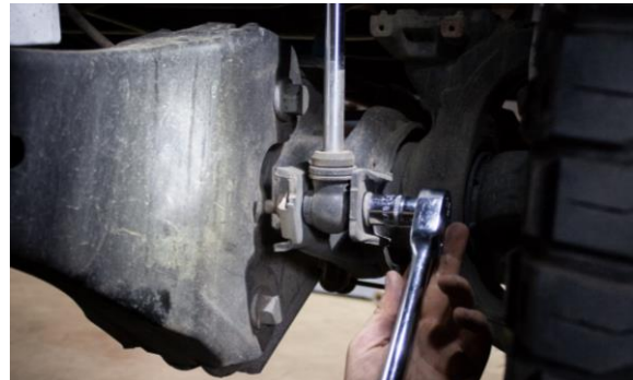
Figure 8B: Front Shock, Lower Mount
