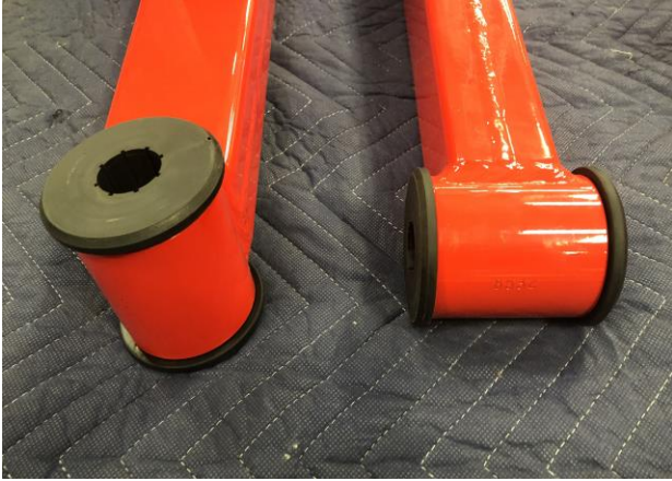
Figure 28: Traction Bar Bushings Installed
